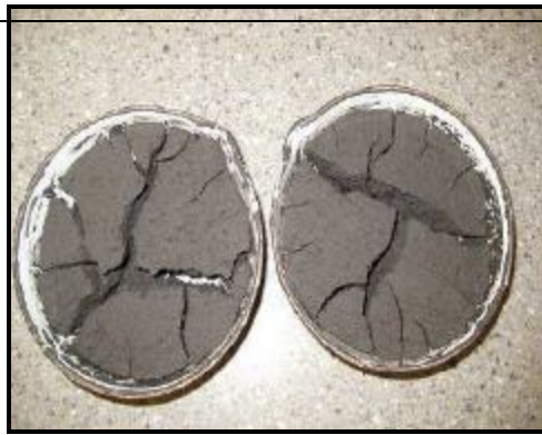
Cracking pattern test
